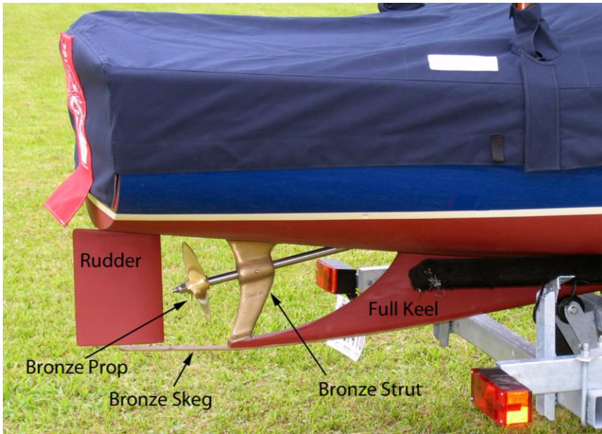
Full keel protection for running gear
